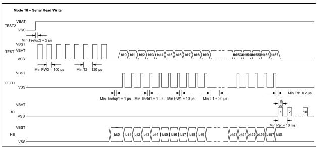
FIGURE 4-7: Timing Diagram for Mode T8.
