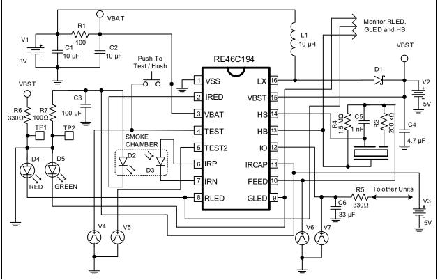
FIGURE 4-5: Circuit for Programming in the Typical Application.
