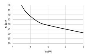
$t_{FALL}~vs.~V_{IN} \label{eq:tfall}$   $(T_A \!=\! +25^{\circ}C,~R_{DIS} \!=\! 1k\Omega,~C_{SS} \!=\! 10nF,~C_L \!=\! 1\mu F,~C_{IN} \!=\! 1\mu F)$
