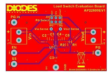
Figure 1. PCB Copper Layout & Silk Screen - Top
