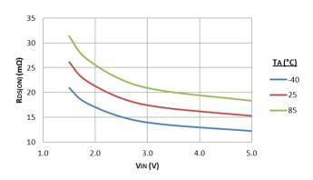
R<sub>DS(ON)</sub> vs. Ambient Temperature (I<sub>OUT</sub>=200mA)
