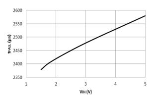
$t_{FALL} \ vs. \ V_{IN}$   $(T_A \! = \! +25^{\circ}C, \, R_{DIS} \! = \! 240\Omega, \, C_{SS} \! = \! 10nF, \, C_L \! = \! 0.1 \mu F, \, C_{IN} \! = \! 1 \mu F)$
